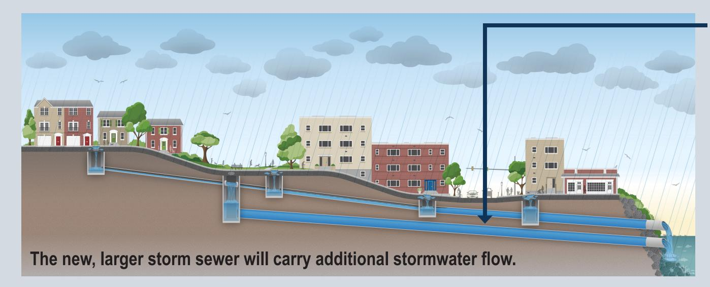
A new and larger-capacity storm sewer will provide an additional route for stormwater to drain. This extra capacity will relieve the existing pipe and mitigate flooding on the road.
